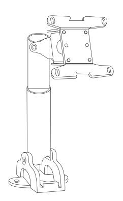
Typical Pedestal Type Mount with Swivel Bracket
